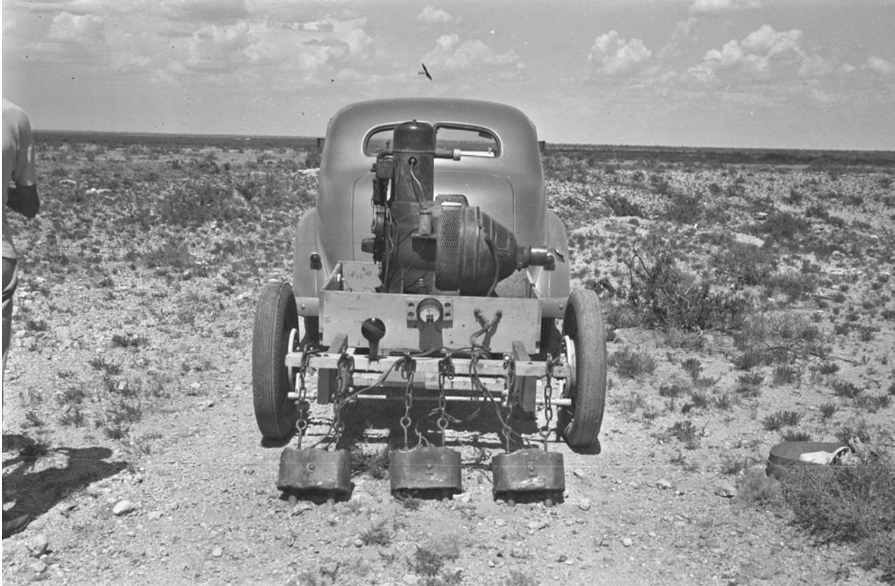
Figure 8. Field vehicle used by Harvey Nininger to search for meteorites in the American West. He attached large magnets to the back, which dragged on the ground to pick up specimens. Photo: H. Nininger.
