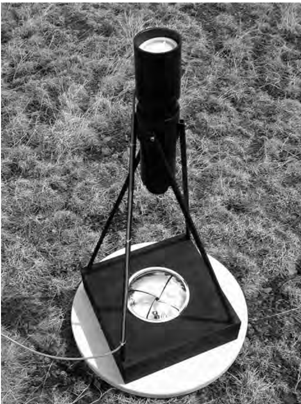
Figure 10. Early prototype of roof-mounted camera and parabolic mirror used to capture images of meteorites entering our atmosphere. Instrument is ~1 m tall. Photo: C. Peterson.
