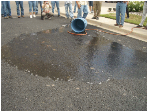
Porous Asphalt, Colorado Stormater Assoc.
